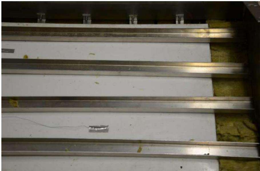
**Figure 4-7. Metallic support bars on the back of the cavity**
