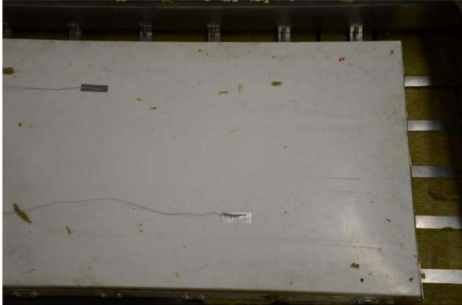
**Figure 4-8. Cavity back plate with thermocouples**
