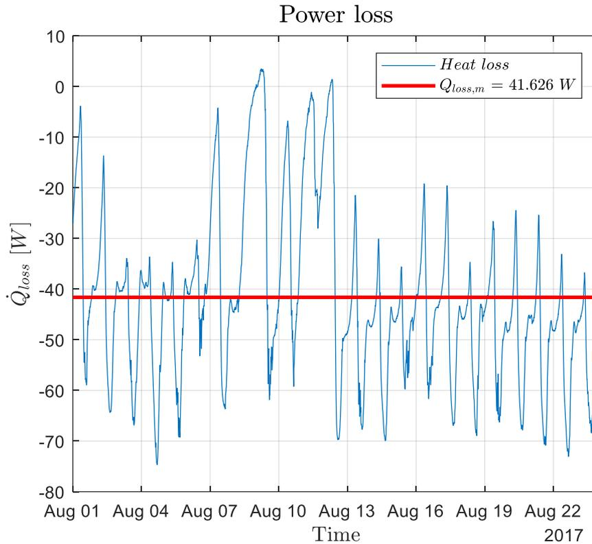
**Figure 3-11. Thermal power loss in August 2017**
